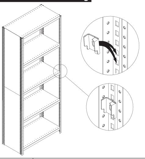
For added strength, place two 1/4-20 x 5/8" bolts and nuts (not included) through each corner of each shelf, and into the small holes of the upright.
