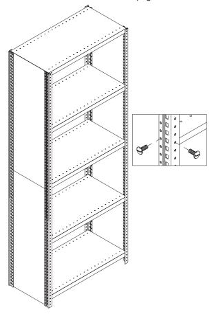
If more than one unit is to be used in a row, assemble a new unit end, and then connect this new end to the existing unit (which you already built with the proper uprights if you followed the instructions in step 2) with a top and bottom shelf. After the end is connected, you can then insert the back by bending it slightly and wedging it between the posts and the shelves. Bolt in place the same as you did for the first unit. Once the
