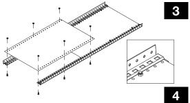
Bolt the panels into the small holes near the edge of both uprights using 1/4-20 x 5/8" bolts and nuts. Leave 16 or 17 holes (16 or 17 inches) between each bolt, as shown in the drawing. Also, if you can predetermine where you want your shelf levels to be, try to position the bolts where they will not interfere with the shelves; this will avoid having to move them later. Finger tighten only at this point, as binding may occur during shelf placement if side panels are attached too tightly.
