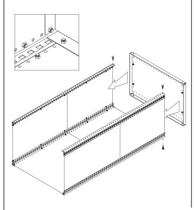
8 Bolt the bottom shelf using the third hole from the
